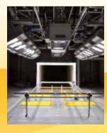
Atlas Custom Systems designs and builds custom solar simulation systems such as walk-in chambers or full-scale test facilities. These full scale test facilities use a series of highly coordinated metal halide lights to provide uniform radiant energy to meet the demanding testing needs of many industries.
