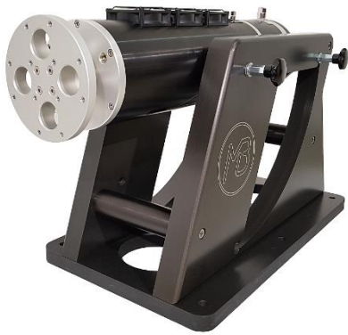
Picture 8: Trunnion base allows quick and easy change between vertical and horizontal orientation of the ALPHA shaker
