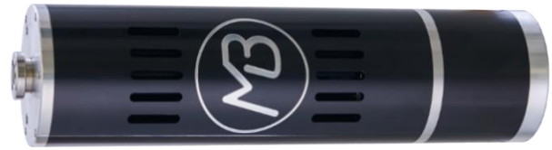
Picture 1: With a weight of only 39kg and a diameter of 198mm the ALPHA 3025 generates excitation forces of 3000N sine peak and instantaneous peak forces of up to 6000N peak. A centric M12 thread allows easy connection to a wide range of test tables and structures.
