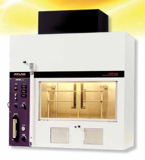
Atlas' HVFAA Horizontal Vertical Flame Chamber accurately determines the flammability of aircraft cabin compartment materials and electric wire. The chamber is designed to perform Tirrill Bunsen burner tests in accordance with FAA's Aircraft Material Fire Test Handbook, Revision 3, DOT/FAA/TC-17/55, chapters A1, C1, D1, D2, and D8 (FAR 25.853, 25.855, 25.1359).
