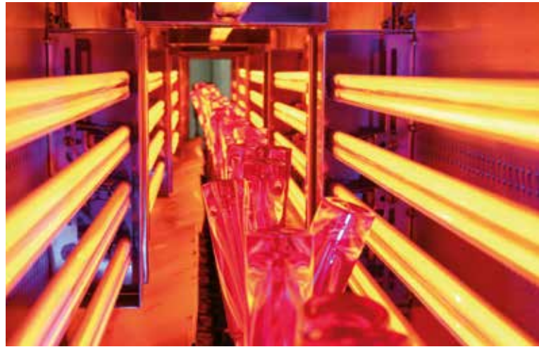
Curing of coatings on glass bottles
